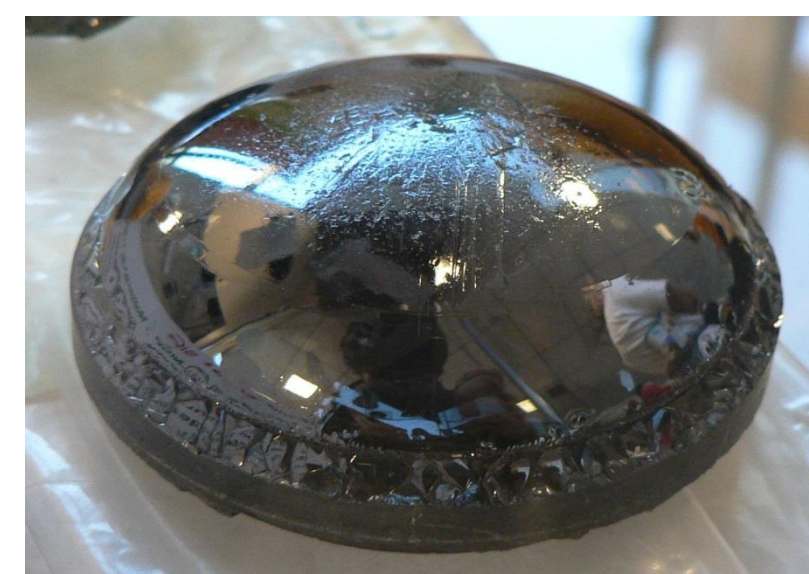
Figure 2 – "Blob" of Silicon Carbide
